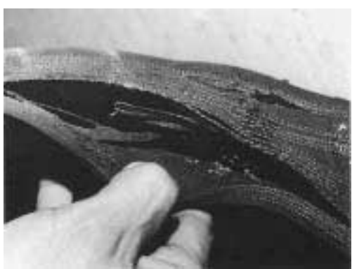
An example of Casing Break Up (CBU) in a bias tire at the lower sidewall caused by running the tire at pressures below those recommended.
